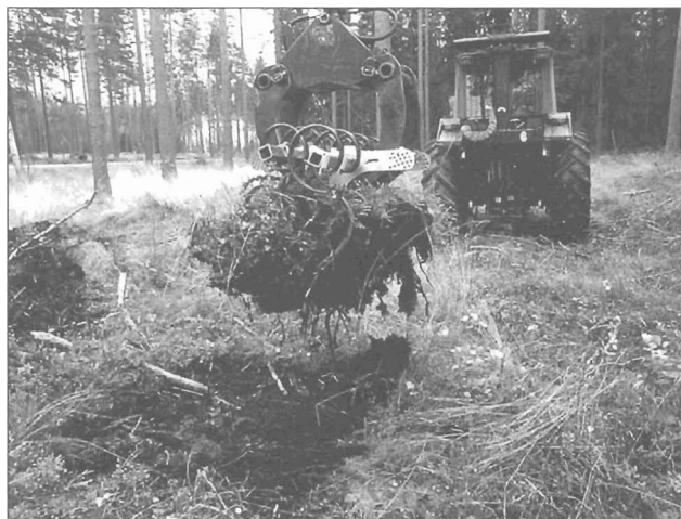
Figure 1. Studied equipment for soil scarification and sowing mounted on a grapple
